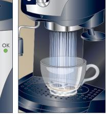
Wait until water is delivered, then turn dial to -W- position to stop the flow.
